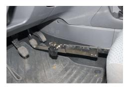
When carrying out leakage checks on the hydraulic brake system it is necessary to maintain a constant brake-pedal pressure over a long period. Constant brake-pedal pressure is also needed to check and adjust brake-pressure regulators or limiters. The ATE pedal arrester is ideal for this purpose.
