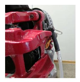
The ATE 90° bleeding hose is a helpful accessory for bleeding in tight spaces. Thanks to its short design, the adapter is only 19 mm in size and allows brake fluid to be removed in spots which are difficult to access.
