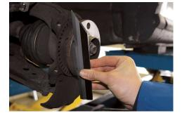
Before a brake disk is mounted, the wheel hub should be checked for flatness (distortion). This is easily done with the ATE straight edge, and the light gap method. Its length of 200 mm allows even larger surfaces to be easily checked.
