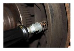
The ATE spring mounting tool is used for the safe and problem-free removal and mounting of the retaining plates of brake-shoe retaining springs. Two different size seating bells safely accommodate large and small spring plates of the brake-shoe retaining springs.
