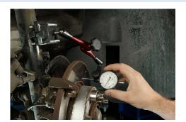
The ATE spacer discs make fast and secure fastening of the brake disc on the wheel hub possible. Using original wheel bolts or nuts up to M14 with spherical or tapered collar, the brake disc is fastened professionally on the hub and prepared for the measurement of axial and radial runout.
