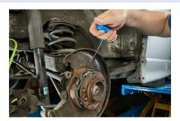
The ATE spring hook is the ideal tool for the straightforward removal and fitting of brake pad retaining springs.
