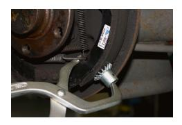
The ATE brake-spring pliers (small) allow the brake shoe return springs on drum brakes to be removed and mounted very easily and safely. The swiveling support plate has sharp claws to provide firm support on the brake lining surface. The hook allows the springs to be attached safely.
