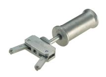
Order no: 03.9314-6100.3 Short order no: 760073 The ATE brake pad withdrawal tool removes firmly seated disk brake pads with retaining holed from fixed calipers. It prevents damage to brake calipers and disks. The fact that the pulling rod is integrated into the sliding weight means that there is no risk of injury.
