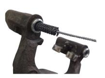
Lubricated guide pins are used to hold the "LUCAS" floating calipers in place. Rubber bellows provide the pin seal. Damaged bellows will make the guide bushes inside the brake caliper holder corrode. This will restrict caliper guide movements and may lead to additional braking problems.
