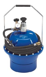
Order no: 03.9302-1350.4 Short order no: 740230 The ATE FB 5p is a pneumatically operated bleeding unit for 5 liters of brake fluid. With the wide range of ATE accessories, all hydraulic clutch and brake systems - including ABS, EDS or ESP - can be filled, flushed and bled. A low-pressure leakage test of a brake or clutch system can also be easily carried out. Only one person is needed to operate the ATE FB 5p.
