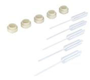
Order no: 03.9311-0019.2 Short order no: 730066 The disposable pipette is used to extract the brake fluid being tested from the vehicle and fill it into the disposable specimen vial so that the boiling point can be determined with the ATE BFCS 300.
