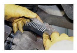
The ATE special wire brush is used to remove slight soiling on the brake pad guide surfaces of brake calipers and holders.
