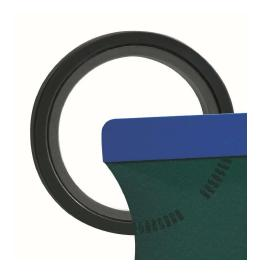
The new active wheel speed sensors work with magnetic sensor wheels, which are integrated in the rubber sealing ring of the wheel bearing. For this, the rubber is enriched with iron dust and then given magnetic fields which are highly sensitive. It is not possible the check the magnetic sensor wheels visually.
