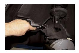
The special ATE bleed wrenches are ring wrenches with an internal hexagonal head to prevent the damage of bleed valves. Thanks to a long offset and a short offset, they can be used without removing the wheel.
