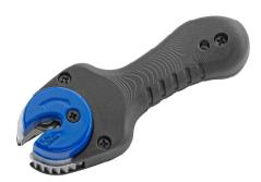
The ATE ratchet pipe cutter is an ideal tool for professionally cutting brake pipes with a diameter of 4.75 mm. Thanks to its compact design and ratchet function, it can be used directly at the vehicle even where space is very tight. The automatic readjustment function means there is no need to retighten the cutting wheel during the cutting process. Only a little force is necessary thanks to the additional leverage provided by the handle length.
