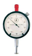
Order no: 03.9304-0034.2 Short order no: 760093 The ATE dial gauge with 1/100 mm reading accuracy is used to measure brake disks and wheel hubs. If measurement is to be carried out in situ on the vehicle, an ATE dial-gauge holder is required.
