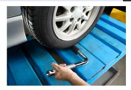
The chassis tester is a simple but very effective aid for localising bearing play in the area of the vehicle axles.
