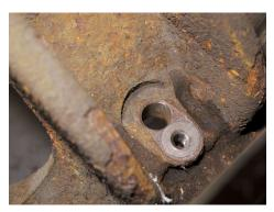
Before the installation of a new ABS wheel speed sensor the mounting hole must be cleaned and returned to nominal size.
