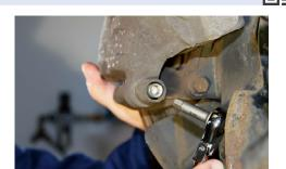
Space is often at a premium around the brake calipers. Conventional tools are hard put to loosen and tighten the guide pins.
