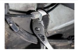
The ATE special grip pliers is the ideal pliers for loosening damaged screw/bolt heads, nuts and studs.
