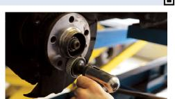
ATE's wheel hub cleaning set 4 is an ideal tool that allows you to clean heavily soiled or slightly rusting wheel hubs quickly, safely and at low cost. Before installing a new brake disc the hub mounting face must be cleaned to bare metal. This is the only way of complying with mounting tolerances and avoiding brake judder.
