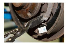
The ATE parking brake cable spring pliers allow simple and safe attachment of the parking brake cable to the brake shoe lever on drum brakes. It is particularly useful for mounting the ATE top kit.
